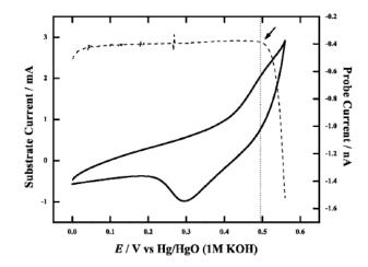
Figure 5. SG-TC SECM measurements (— CV, — probe current) of 100  $\mu$ m coating of nickel hydroxide (type A) standard mix (active material, graphite, and binder) on 20  $\mu$ m nickel foil at a scan rate of 2 mV s<sup>-1</sup>. The arrow indicates the point of oxygen detection at the probe tip.
