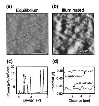
SKP area maps and line scans of p-type GaN w/o and under illumination. Illumination reduces the overall surface potential and increases the magnitude of surface potential variations.
