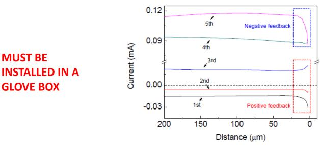
Figure 1. Current profiles measured by PSC technique. (potential conditions are 0.0V for Li metal tip and 4.0V for Pt electrode)
