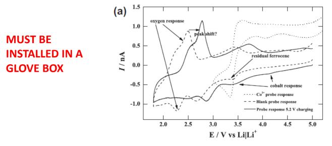
Cyclic voltammogram of the Pt (10 lm) microelectrode probe tip in C4mpyrTFSI at 50 mV s-1, showing the effect of overcharging by utilising a bias potential of 5.2 V vs Li|Li+
