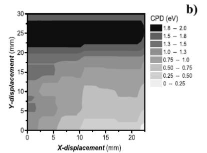
Contact Potential (or Work Function) Difference map of a multicrystalline Si, Bdoped, NaOH etched wafer.
